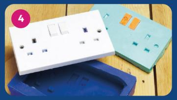
You can demould in as little as 20 minutes dependent on the thickness of your Body Double mould. You can now cast numerous materials into the mould such as Fast Cast resin, plaster, wax and low melt alloys.
