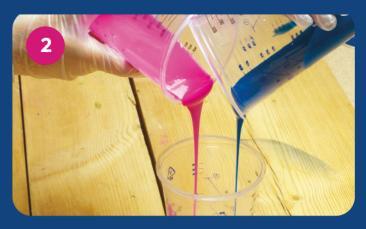
Body Double comes in two parts with mixing ratios of 1:1. Using accurate measuring cups, pour an equal measure of Part A into one cup and do the same for Part B in another cup. Pour both cups into a third cup. Ensure the two coloured components are mixed thoroughly so that they can create a uniform purple liquid. You now have a working time of approximately six minutes.
