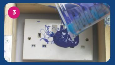
Working quickly, coat your object with Body Double. You can pour Body Double onto the object or brush it on using an ordinary, good quality brush. Remember to leave enough area uncoated to allow casting materials to be poured in.
